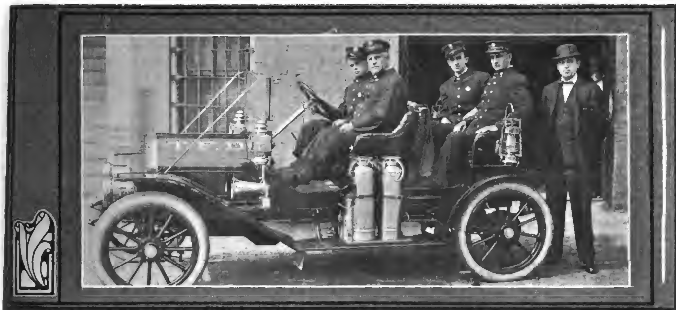
Fig. 8—E-M-F car used at Taunton, Mass., showing a chemical equipment on the running board; also the chief and company.
